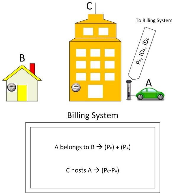
Figure 2: Separate billing using CMS
